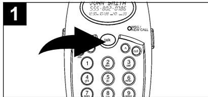
**1** After the battery has been fully charged, press the TALK button and listen for a dial tone; the IN USE indicator on the base will light and "TALK" as well as the timer will appear on the display.
