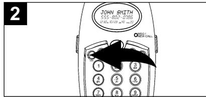
2 Press the OPTION button repeatedly until the desired prefixes appear. If a 1 in the area code is necessary to dial, then press the OPTION button repeatedly until the 1 and the area code appear before the number.
