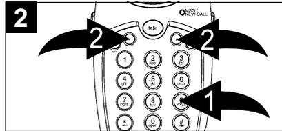
2 Press the Key button 9 <sup>1</sup>, or the Up/Down buttons <sup>2</sup> to select the Pause Time setting.
