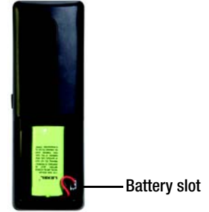
Figure 3-3: Battery pack installed
