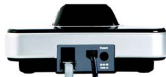
Figure 3-1: Telephone cable connection
