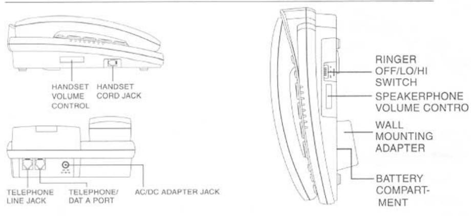
AC ADAPTER FOR DC JACK SPECIFICA TION OUTPUT-DC 9V. 100 mA POLARITY OF PLUG
