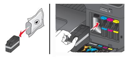
**Note:** Install the new ink cartridges immediately after removing them from the packaging to avoid exposing the ink to air.
