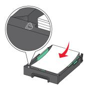
**5** Adjust the paper guides to rest against the left, right, and bottom edges of the paper.
