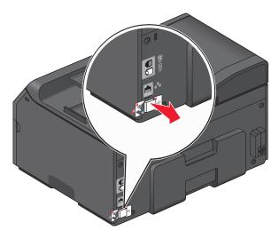
2 Firmly plug the square end of the USB cable into the back of the printer.
