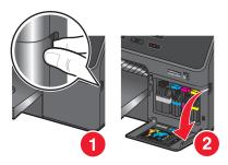
**Warning—Potential Damage:** Do not extend the ink cartridge access door beyond 90 degrees when opening to prevent it from breaking.
