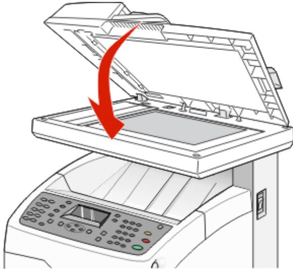
7 When all the jammed paper is removed, **Return the Removed Original and Press Start** appears. Place the original document in the ADF, and then press **Start**
