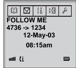
The display shows your own extension number 4736 diverted to the desired diversion target.
