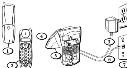
Because it is necessary to charge the handset for 12 hours prior to connecting the phone for use the first time, it is better to leave the unit on a flat surface during initial charge before attempting to hang it on the wall.
