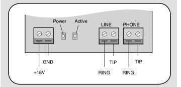
Use the supplied Test/Program Cord for programming and testing before completing connections to phone company's de-mark box.
