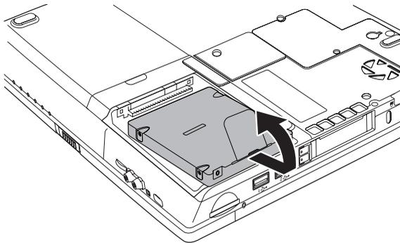
Figure 8-17 Removing the HDD pack
