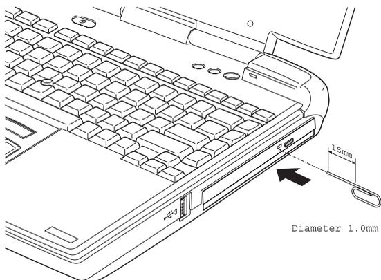
*Figure 4-7 Manual release with the eject hole*
