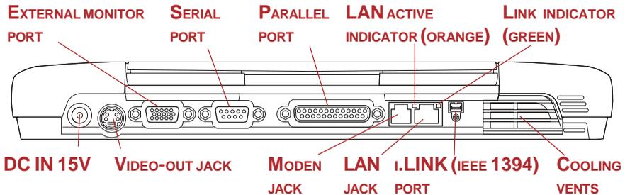
Figure 2-4 The back side of the computer
