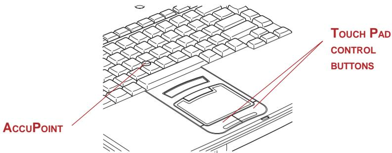
Figure 4-1 Touch Pad and Touch Pad control buttons
