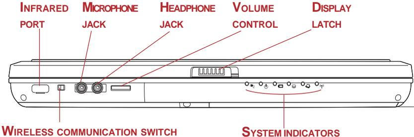
Figure 2-1 Front of the computer with display closed
