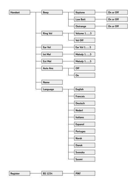
**Important.** If you make a mistake you can return to the previous menu heading by pressing the  $\bigstar$  button. If you press and hold the  $\bigstar$  button at any time you will return to the standby screen. After 15 seconds if no buttons are pressed the handset will automatically return to the standby screen.
