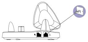
Do **not** connect the other end to the wall socket until at least one handset is fully charged.
