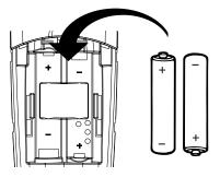
Slide the battery compartment cover back into place.
