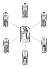
Each handset can be registered on up to four bases.
