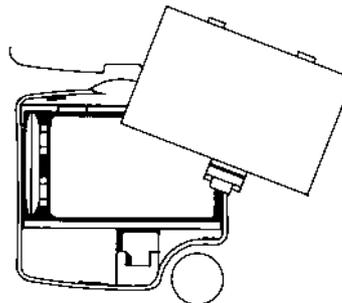
The back-up battery is available separately and ensures your Freestyle 1050 retains messages, settings and stored phone numbers if there is a mains power failure. If no battery is installed, the **BATT LOW** light comes on when the mains power is switched on.
