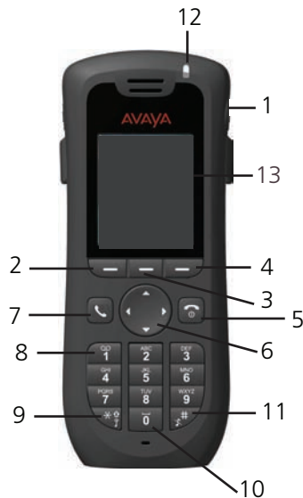
Figure 1: Description of the cordless telephone
