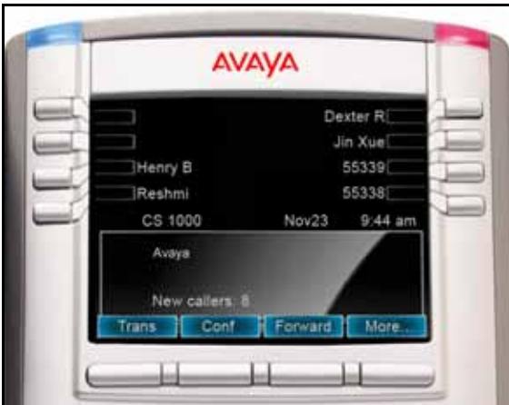
Figure 34: Logged in to an Avaya 1165E IP Deskphone
