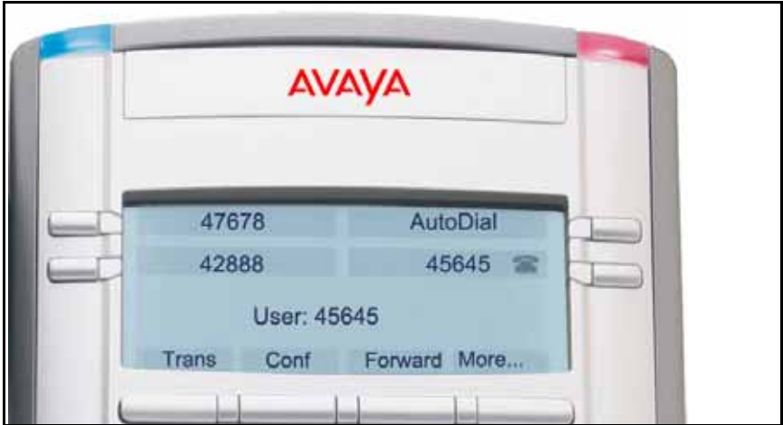
Figure 35: Logged in to an Avaya 1165E IP Deskphone using an Avaya1120E IP Deskphone
