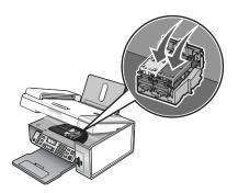
5 Close the scanner unit, making sure to keep your hands out from underneath the scanner unit.
