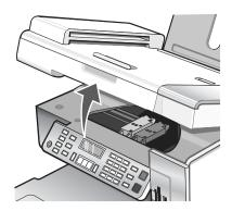
3 Press down on the cartridge carrier lever to raise the cartridge carrier lid.
