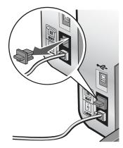
4 Connect the other telephone cord to a telephone, and then plug it into the EXT port in of the printer.
