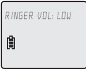
1. Press and hold **▼CID** or **DIR ▲** when the cordless handset is idle (not in use). This feature allows you to choose low, med, high ringer volume or turn the ringer off.
