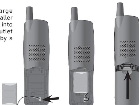
3. Insert the plug as indicated. Be sure to securely insert the plug, making sure matches the color-coded label inside the battery compartment.
