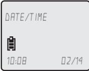
Each cordless handset operates individually from the other handsets. The ringer sound, ringer volume, date & time, dial mode and language must be programmed separately for each cordless handset. Follow the steps below to program the cordless handset. To stop at any time, press **OFF/CLEAR**.
