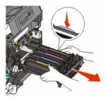
**8** Remove the used developer unit.
