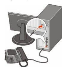
**5** Connect a third telephone cord from the computer modem to the bottom EXT port **1** of the printer.
