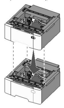
**4** Align the printer with the 650-sheet duo drawer, then lower the printer into place and install the dust covers.
