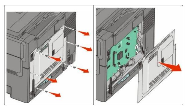
**Warning—Potential Damage:** System board electronic components are easily damaged by static electricity. Touch something metal on the printer before touching any system board electronic components or connectors.
