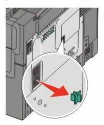
**2** Connect your telecommunications equipment directly to the bottom EXT port **a** on the back of the printer.
