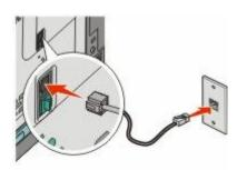
**3** Remove the protective plug from the bottom EXT port **a** of the printer.
