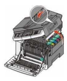
Remove the toner cartridges by lifting the handles and then gently pulling away from the imaging kit.
