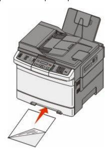
**Note:** Align the long edge of the print media so that it is flush with the right side of the manual feeder.
