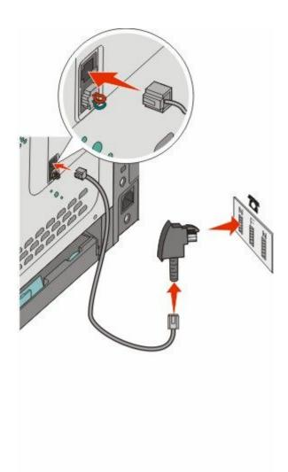
**3** If you would like to use the same line for both fax and telephone communication, then connect a second telephone line (not provided) between the telephone and the F slot of an active analog telephone wall jack.
