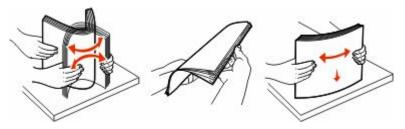
• Hold transparencies by the edges and fan them. Straighten the edges on a level surface.
