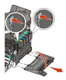
Press the green levers on each side of the waste toner bottle, and then remove it.
