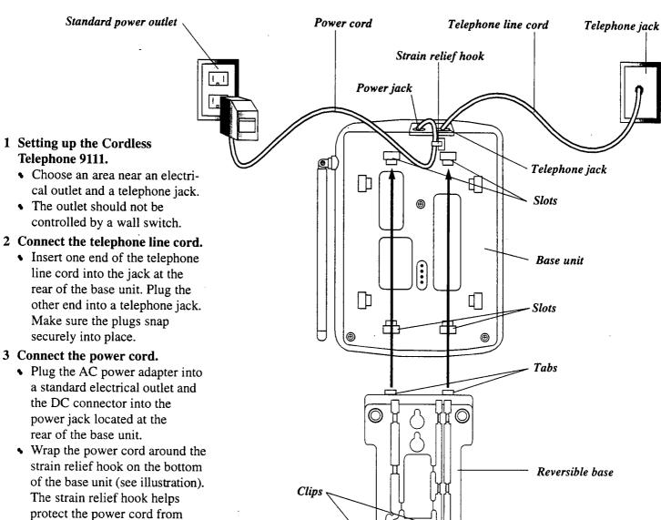
CAUTION: Use only the AC power adapter supplied with this telephone. This is a Class 2 AC adapter, specifically designed for use with the 9111.
