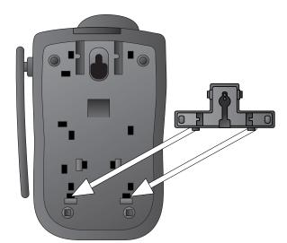
Align tabs on wall mount adapter with holes on bottom of base. Snap wall mount adapter firmly into place.
