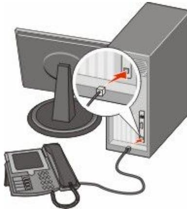
**5** Connect a third telephone cord from the computer modem to the bottom EXT port
