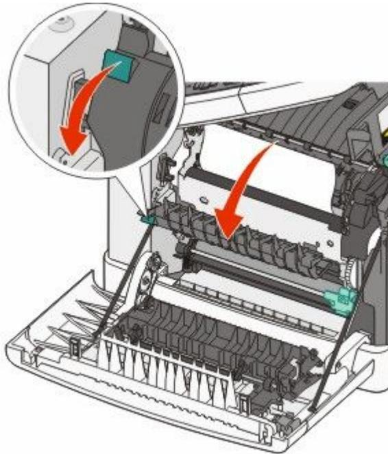
3 Hold the fuser cover down, and then remove the jammed paper.
