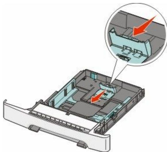
**Note:** Use the size indicators on the bottom of the tray to help position the guide.
