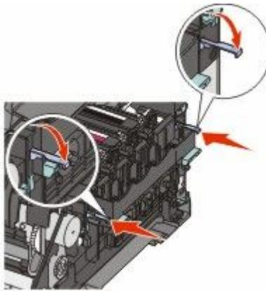
**16** Rotate the blue levers down until the imaging kit drops into place.
