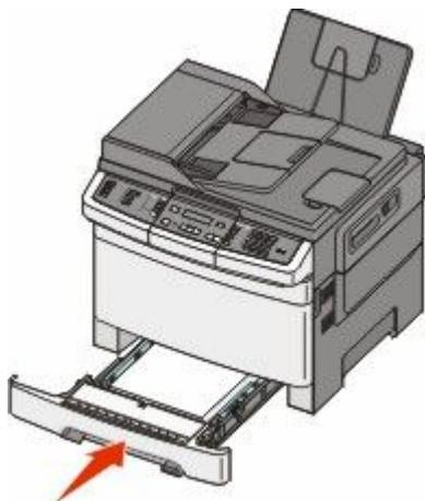
8 If a different type or size of paper was loaded than the type or size previously loaded in the tray, change the Paper Type or Paper Size setting for the tray from the printer control panel.
