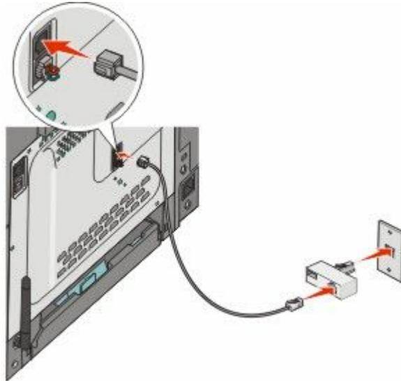
**3** Connect the answering machine or telephone to the adapter
