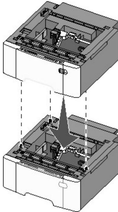
4 Align the printer with the 650-sheet duo drawer, then lower the printer into place and install the dust covers.
