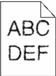
If you are using downloaded fonts, verify that the fonts are supported by the printer, the host computer, and the software program.
