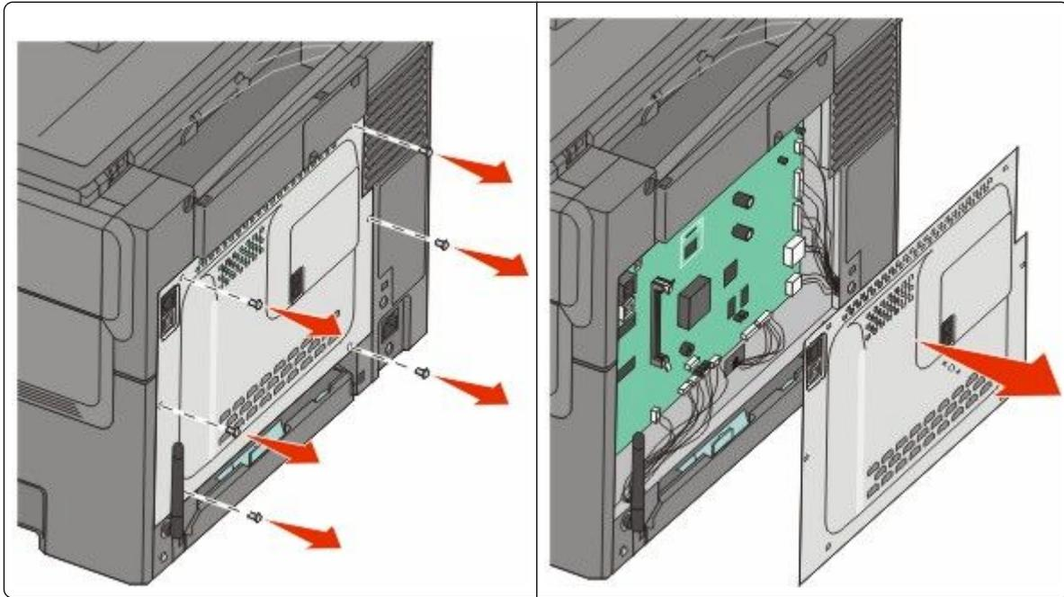
**Warning—Potential Damage:** System board electronic components are easily damaged by static electricity. Touch something metal on the printer before touching any system board electronic components or connectors.
