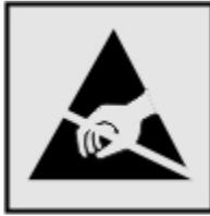
This symbol identifies static-sensitive parts. Do not touch in the areas near these symbols without first touching the metal frame of the printer.
