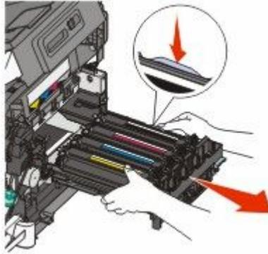
8 Remove the used developer unit.
