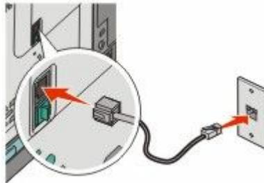
**3** Remove the protective plug from the bottom EXT port
