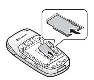
4. Place the battery so that the 3 brass tabs on the end align with the 3 brass prongs at the bottom of the battery compartment (1). Press the battery down until it clicks into place (2).
