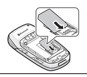
Note: If you need to remove the SIM card, slide it, as shown, and take it out of the socket.
