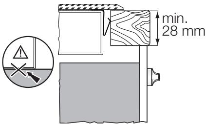
**i** If you use a protection box (the additional accessory), the protective floor directly below the appliance is not necessary.
