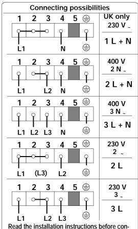
Read the installation instructions before connecting the mains cable. Ensuring that the links are fitted correctly to the terminal block
