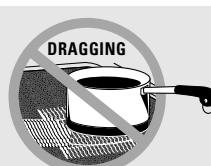
Do not slide cookware across the control or cooktop surface because it can scratch the glass. The glass is scratch-resistant, not scratchproof.
