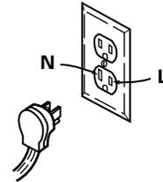
Ensure proper ground and firm connection before use
