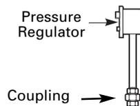
To reduce the likelihood of gas leaks, apply teflon tape or a thread compound approved for use with LP or Natural gases to all threaded connections.
