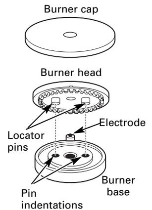
Make sure the slot in the burner head is positioned over the electrode. The burner cap has three to four pins. When replacing the cap, make sure none of the pins sits in the stability chamber.
