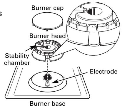
Make sure the hole in the burner head assembly is positioned over the electrode and that the burner head is fully inserted inside the burner base. A small gap between the base and head is normal.
