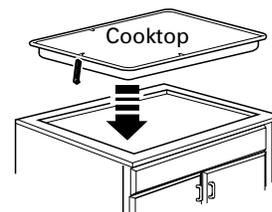
Once the unit is in place, screw the hold-down bracket into the cabinet sides to secure the unit into place.
