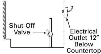
Install a manual shut-off valve in the gas line in an easily accessible location outside the cooktop. Be sure you know how and where to shut off the gas supply to the cooktop. Install the electrical outlet 12" below the countertop.
