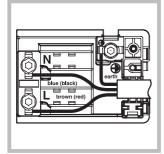
3 Remove the wire contact screws L-N- $\pm$ , then fasten the wires under the screw heads, respecting the colour code: Black/Blue (N), Red/Brown (L) and Bare Wire/ Yellow-Green ( $\pm$ ).
