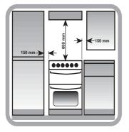
The height of the cooker can be adjusted by means of adjustable feet in the plinth (900mm - 930mm). Adjust the feet by tilting the cooker from the side. Then install the product into position.
