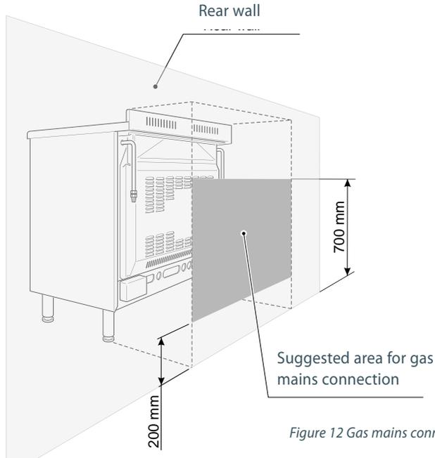
Figure 12 Gas mains connection area
