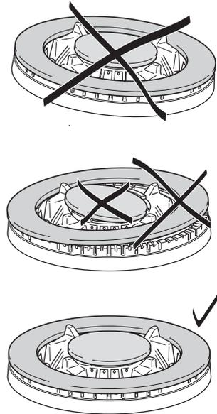
Figure 35 Replacing the triple ring wok burner
