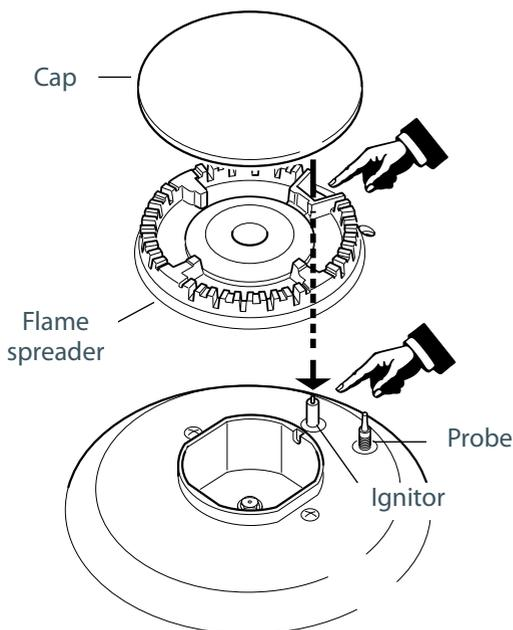
Figure 32 Auxiliary, rapid and semi-rapid burner parts
