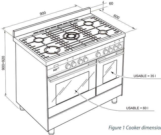
Figure 1 Cooker dimensions and capacity
