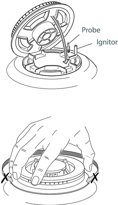
Figure 34 Triple ring wok burner parts
