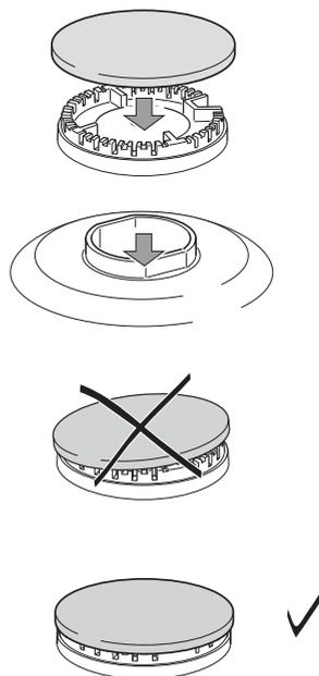
Figure 33 Replacing the auxiliary, rapid and semi-rapid burners
