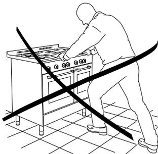
Figure 7 Incorrectly moving the cooker
