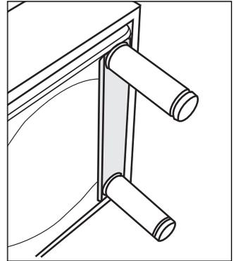
Figure 4 Top of feet screwed in tightly
