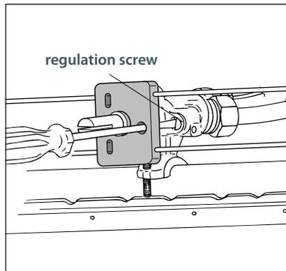
Figure 15 Adjusting the minimum burner setting
