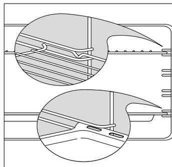
Figure 29 Correct position of shelves and pan
