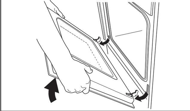
4. place the oven door on a solid surface, being careful to avoid the glass becoming scratched. Then remove the two screws located on the sides of the oven door;
