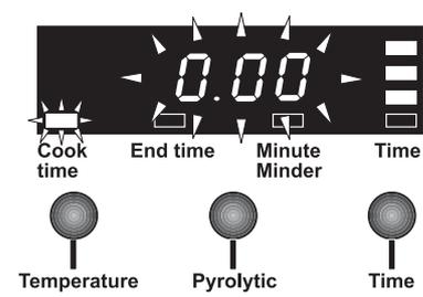
**i** If you turn the oven knob to a cooking function while the pyrolytic function is active, the cleaning cycle will be interrupted.
