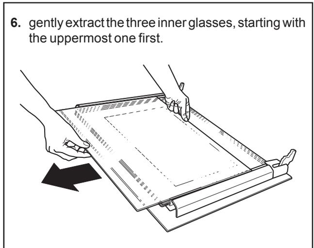
Clean the oven door glass with warm water and a soft cloth only. Never use harsh abrasives as they could damage the special heat-resistant surface of the inner glasses. Once the cleaning is carried out, refit the oven door following the procedure in reverse.
