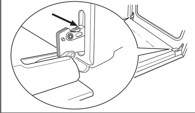
2. unlock and turn the small levers located on the two hinges;
