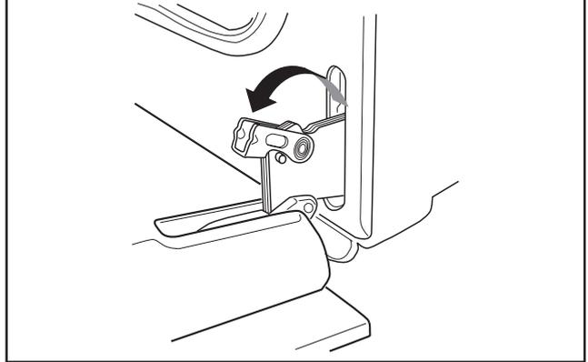
3. handle the door by its left- and right-hand sides, then slowly turn it towards the oven until it is half-closed; at this point, gently pull the oven door away from the oven frame;
