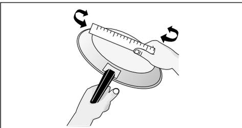
Pans should have flat bottoms. Check for flatness by rotating a ruler across the bottom. There should be no gaps between the pan and ruler.
