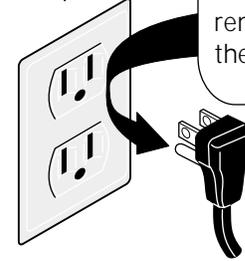
Power supply cord with 3-prong grounding plug
