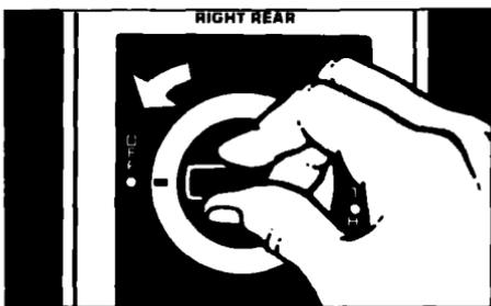
**Control knobs must be pushed in, then turned to the LIGHT position.** On electronic ignitor model, the clicking sound is the ignitor sparking. After the burner lights, turn the control knob back to a desired setting. The control knob can be set anywhere between HI and low setting. **Do not cook with the control in the LIGHT position.**
