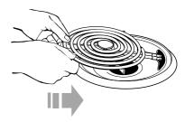
**4.** When the terminal is pushed into the receptacle as far as it will go, push down the edge of the coil element opposite the receptacle.
