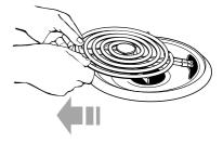
**4.** Lift out the reflector bowl. See the "Cleaning chart" later in this section for cleaning instructions.
