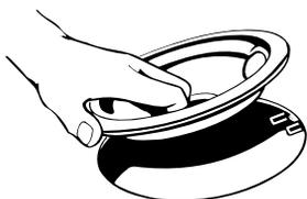
2. Holding the coil element as level as possible, slowly push coil element terminal into the receptacle.
