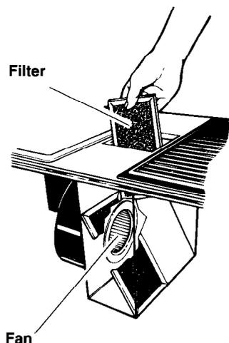
1. Remove the vent cover and wash in warm, soapy water or wipe with a damp cloth. **Do not use metal scrubbing pads or abrasive cleansers.**
