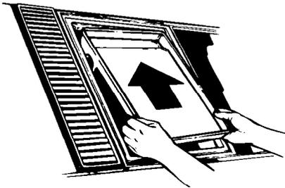
2. Slide the griddle into place with drain slot at rear.
