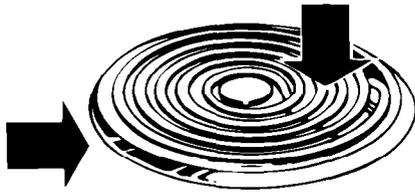
3. While pushing the surface unit terminal into the receptacle, lift a little on the edge of the unit nearest the receptacle.
