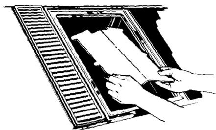
3. Lift out splatter shield.
