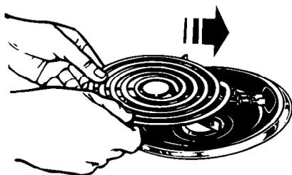
2. Hold the surface unit as level as possible with the terminal just started into the receptacle.
