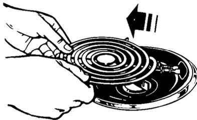
1. Lift the edge of the unit opposite the receptacle, just enough to clear the reflector bowl.
