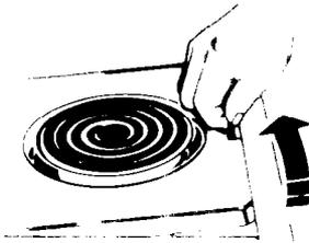
**1. To remove**, lift slightly by the handle.
