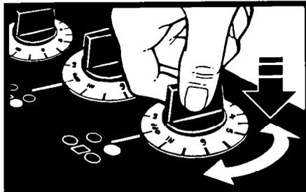
Control knobs must be pushed in before turning them to a setting. They can be set anywhere between HI and OFF.
