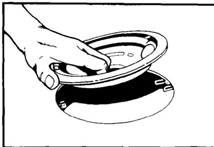
2. Line up openings in the reflector bowl with the surface unit receptacle and the element hold down clip.
