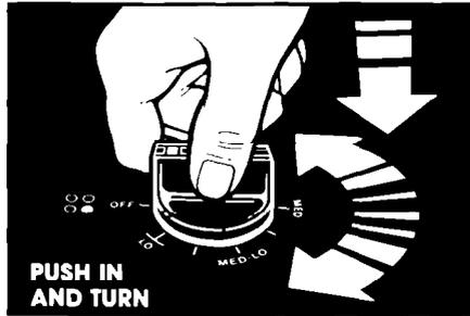
**Control knobs must be pushed in before turning** them to a setting. They can be set anywhere between HI and OFF.
