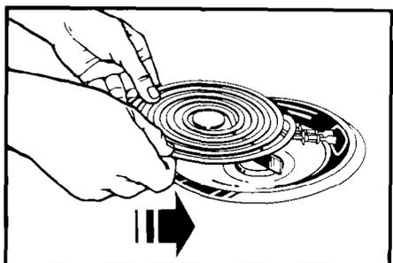
3. Hold the surface unit as level as possible with the terminal just started into the receptacle. Push the surface unit terminal into the receptacle.
