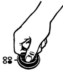
2. **Line up** openings in the drip bowl with the surface unit receptacle and the element hold-down clip.
