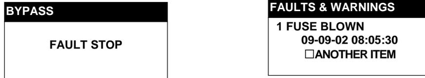
Select the desired fault data with the scroll buttons.
