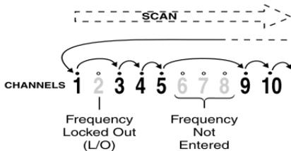
The BC278CLT scans programmed channels at rate of up to 25 channels per second until it locates an active frequency. When the scanning stops on an active frequency, it remains on that channel as long as the transmission continues. When the transmission ends, the scanner stays on the channel for 2 more seconds, waiting for a responding transmission. If no responding transmission is detected, the scanning cycle resumes until another transmission is received (DELAY function).
