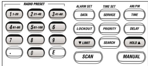
3. Press **AM/PM** to select the desired setting, either a.m. or p.m.
