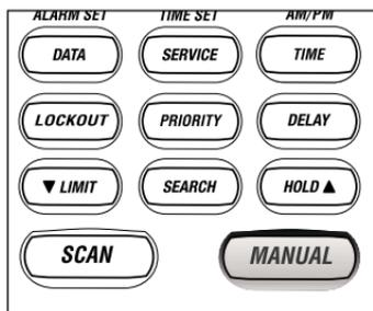
2. To select the channel (12), press **1**, then **2** on the numeric keypad. Then press **MANUAL** again.
