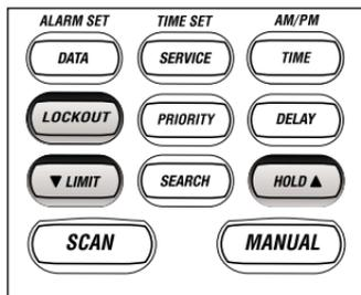
To cancel this function, press **HOLD▲** to hold the search and select the frequency by using **HOLD▲** or **▼LIMIT**, then press **LOCKOUT**.
