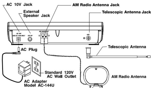
1. Insert the small plug at the end of the AC Adapter cord into the **AC 10V** jack on the scanner.
