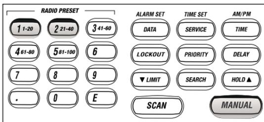
3. Type in the frequency numbers, including the decimal point, using the numeric keypad: 420.0150. Channel digits flash as you make entry.
