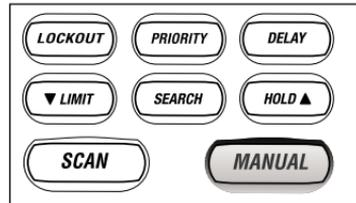
2. Press 5 then **MANUAL** for direct channel access. Or select channel 5 using the ▼ / ▲ keys.
