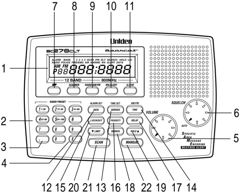
1. **LCD Display** Displays time, channel, frequency, and functions. (Page 6)
