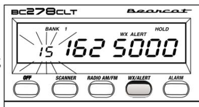
Your scanner now functions as a Weather Alert radio, waiting to receive a severe weather emergency tone. When your scanner receives the emergency tone from your local NOAA weather station, it responds with a loud siren at maximum volume (regardless of the volume control setting). The siren will continue until the emergency tone stops transmitting.
