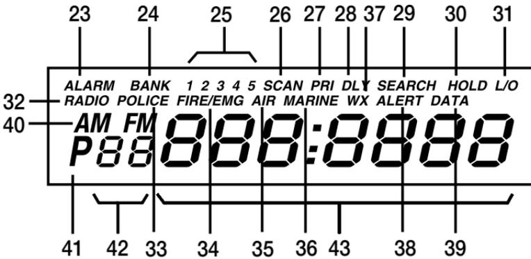
23. **ALARM** Appears when Alarm function is active. Flashes in the snooze function mode.
