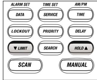
2. Press **HOLD▲** to move to the next higher frequency, or press **▼LIMIT** to move down to the previous frequency.
