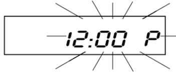
2. Then enter the time directly by pressing the numeric keys.
