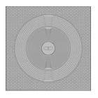
The dual element comprises two cooking zones: an inner one and an outer one. If the size of the pan is the same as the inner cooking zone, it will work as a single element.
