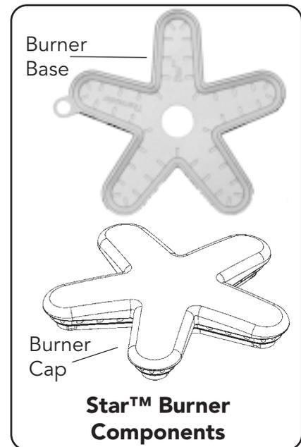
Each burner has its own electronic igniter that sparks when the burner is turned on. Each burner should light in 4 seconds or less. If a burner does not light, check to see that the cap is positioned correctly on the base. **Do not touch the burners when the igniters are sparking.** If a burner fails to ignite, refer to the section on Page 30 "Before Calling for Service."
