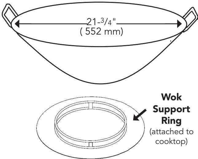
3. Check that the support ring is properly placed above the burner.
