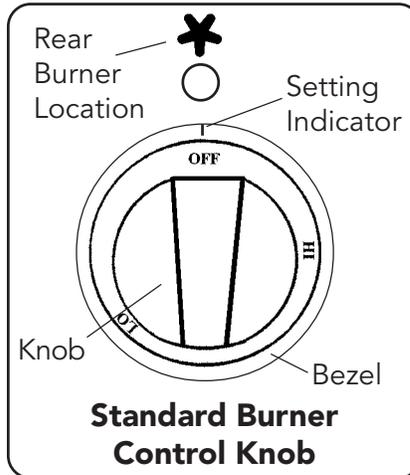
The icon above each control knob shows whether the burner position is in the front or in the rear. A solid star indicates the location of the burner controlled by that particular knob. The drawing above shows the knob controlling the rear burner.
