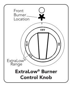
The drawing shows that the control knob has an additional range between the LO and XLO settings. When the knob is set within this range, the flame pulses off and on. By varying the length of time the flame is off and on, the heat is reduced even further to cook delicate foods. For example, these very low settings are suitable for simmering and poaching, melting chocolate and butter, holding cooked foods at temperatures without scorching or burning, etc.
