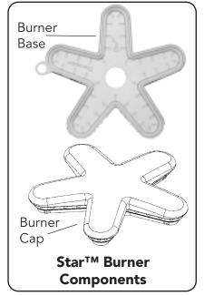
Each burner has its own electronic igniter that sparks when the burner is turned on. Each burner should light in 4 seconds or less. If a burner does not light, check to see that the cap is positioned correctly on the base. **Do not touch the burners when the igniters are sparking.** If a burner fails to ignite, refer to the section on Page 30 "Before Calling for Service."
