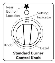
The icon above each control shows whether the burner position is in the front or in the rear. A solid star indicates the location of the burner controlled by that particular knob. The drawing above shows the knob controlling the rear burner.
