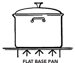
• A heavy, flat base is more apt to remain flat when heated. Pan bases that are warped, dented, ridged or too lightweight will heat unevenly. Heat and cool pans gradually to avoid sudden temperature changes which tend to distort cookware. Do not add cold water to a hot pan.
