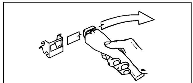
To correctly locate the grill pan on the shelf, ensure that the cut out on the underside of the handle bracket locates over the front bar of the shelf.
