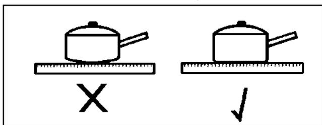
The size of the base of the saucepan should be the same or up to 3cm/1 inch larger than the hotplate. If the base is too small energy will be wasted, boilovers will also be more difficult to deal with as spillage will fall directly onto the hotplate.
