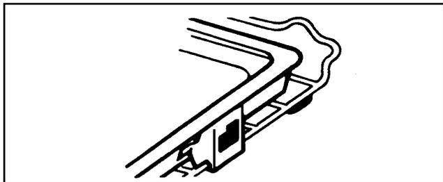
To check the progress of the food being grilled, the grill pan should be withdrawn on the shelf to attend to food during cooking or the carrier shelf can be lifted away from the cooker and rested on a heat resistant work surface.
