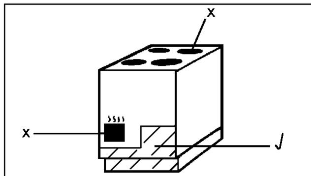
To move the cooker, open the fan oven door, and lift the cooker by holding inside the top of the compartment.
