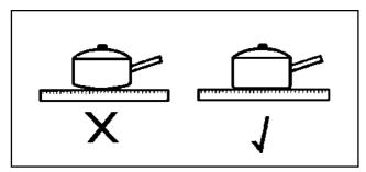
The size of the base of the saucepan should be the same or up to 3cm/1 inch larger than the hotplate. If the base is too small, energy will be wasted, boilovers will also be more difficult to deal with as spillage will fall directly onto the hotplate.
