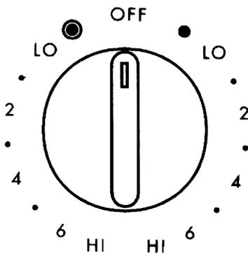
When the elements are turned on, a red glow can be seen through the glass. The elements cycle on and off to keep the selected heat setting. Poor cookware causes the element to cycle on and off more often. (See Temperature Limiters on Page 8).
