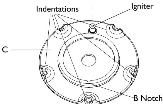
The Burner Cap is porcelain enamel and has a tab (A) on the underside that fits into the notch (B) on the burner base (C). The circle of gas ports are located under the burner cap. If these ports (D) are clogged, use a wire, a straightened paper clip or a needle to clear the ports. Do not use a toothpick; it could break off inside the port. If the condition persists, contact a service agency for adjustment.
