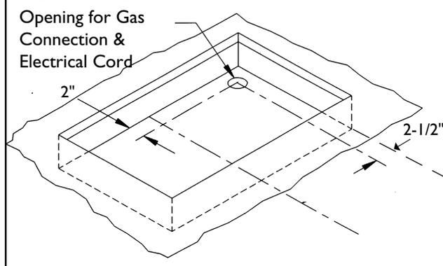
Connect the gas supply line to the unit pressure regulator using a 1/2" flex gas line connector between wall shut-off valve and pressure regulator.
