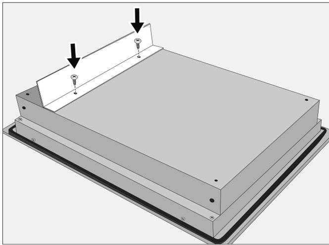
Screw the front heat shield to the base of the burner box using the pre-drilled holes, as shown in the illustration.
