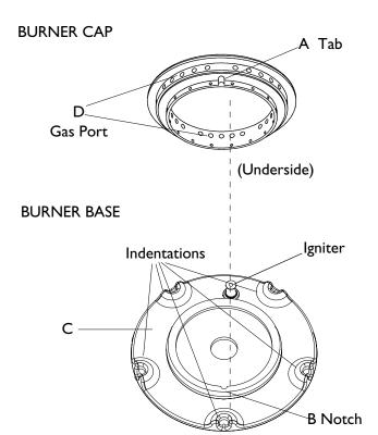
The Burner Cap is porcelain enamel and has a tab (A) on the underside that fits into the notch (B) on the burner base (C). The circle of gas ports are located under the burner cap. If these ports (D) are clogged, use a wire, a straightened paper clip or a needle to clear the ports. Do not use a toothpick; it could break off inside the port. If the condition persists, contact a service agency for adjustment.
