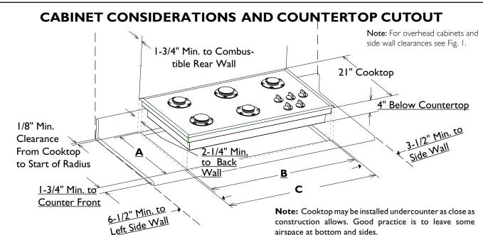
Figure 2 - Cutout Dimensions Are Underlined
