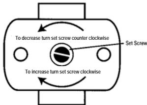
1. Turn off unit and disconnect from electrical power before attempting to adjust the thermostat setting.
