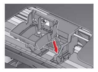
9. Push firmly against the target label of the printhead until you hear a loud snap.
