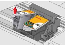
4. Unlatch the printhead by pushing the button in the center of the carriage.
