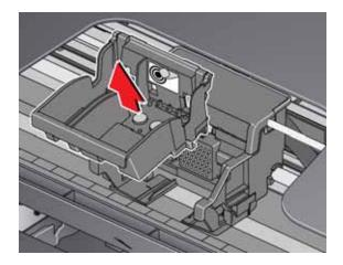
6. Remove the new printhead from its bag.
