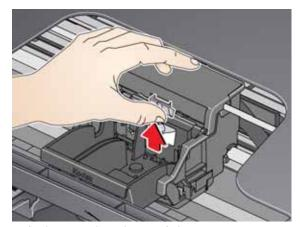
5. Lift the printhead out of the carriage.
