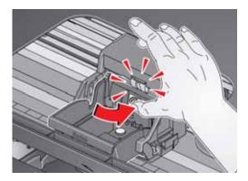
10. Insert the black ink cartridge into the printhead.
